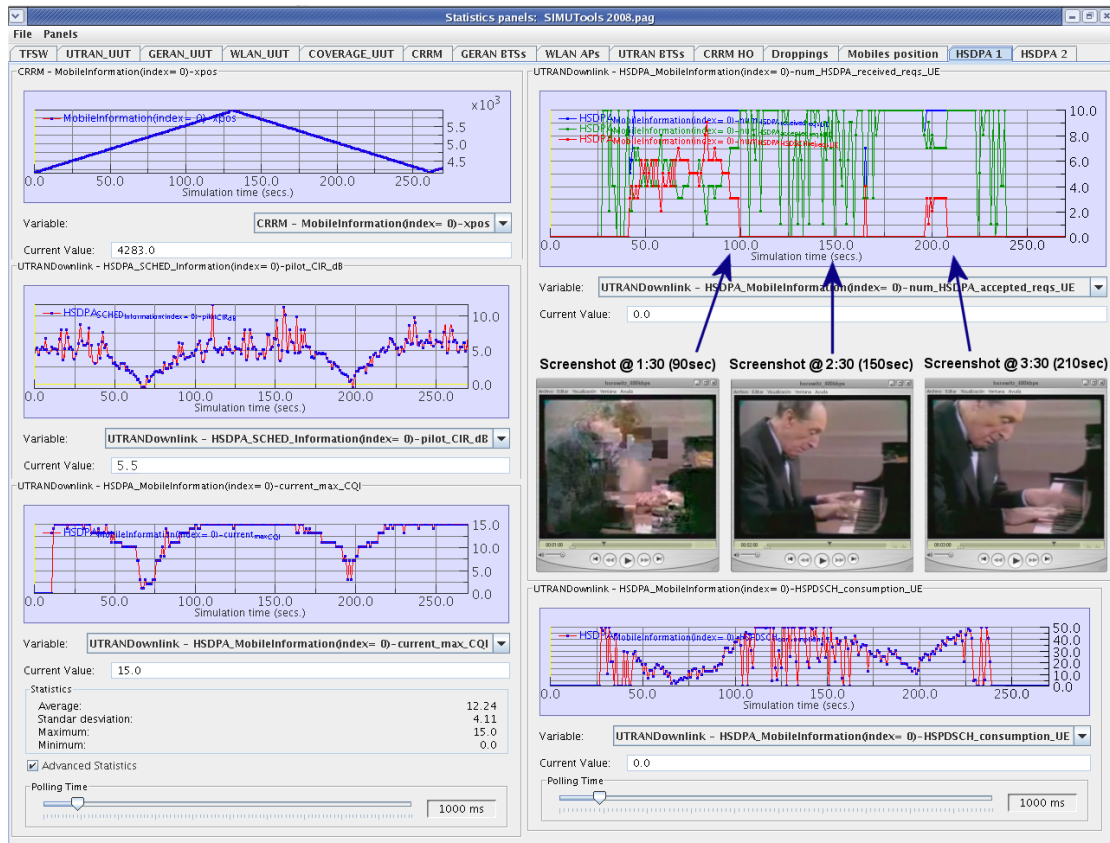
Figure 18. Real-time performance of the Maximum C/I scheduling criterion.
