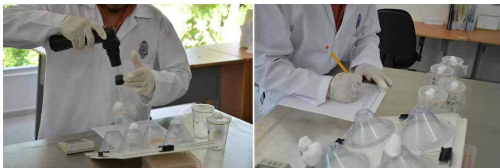
Figure 36. WHO cone test. For evaluate de bioefficacy of LLIS, time-limited exposure tests were carried out. Batches of mosquitoes (5 per cone) were tested on treated netting for 3 min (10 replicates), knockdown scored after 30 min and 1 h and mortality after 24 h.
