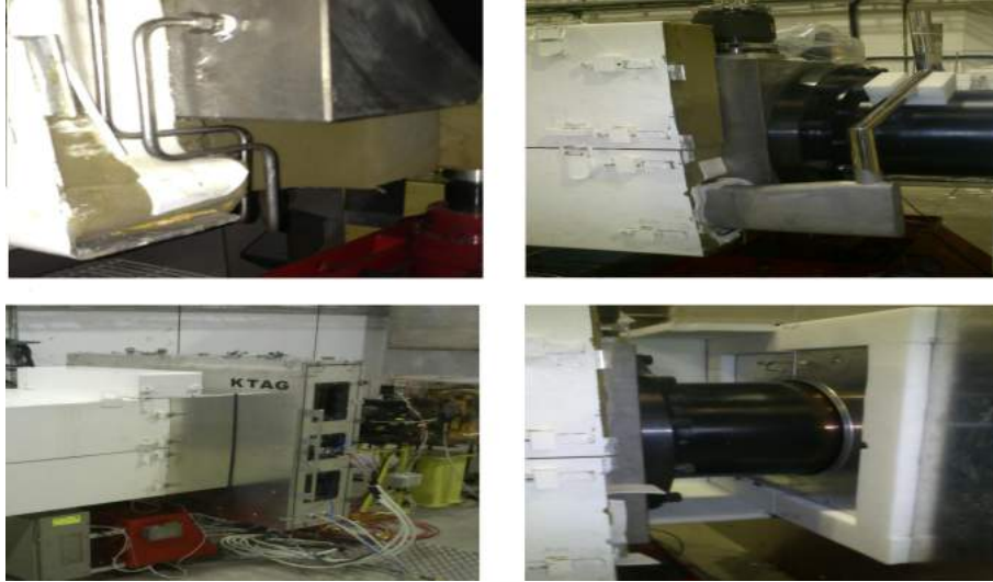
Figure 4.18: Clockwise from the top left. One of the inlet/outlet pipes that need to be covered. One of the two chimneys used to cover the inlet and outlet pipes. One half of the enclosure lined with Rohacell 51S. The full enclosure assembled between CEDAR and KTAG.
