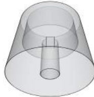
Figure 4.10: A 3D model of the component used to hold a helium laser pointer. It is made so that it fits into the atex cylinder so that we can calibrate the spherical mirror positions.
