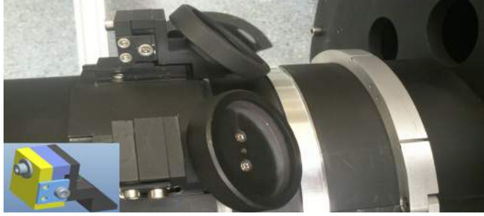
Figure 4.11: The Final stage design installed on the mirror cylinder at Liverpool, calibrated and ready to be shipped to CERN.
