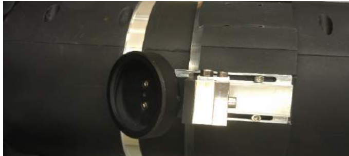
Figure 4.8: Above view of the prototype spherical mirror stage design showing two of the four screws which when loosened allow the z position to be varied.
