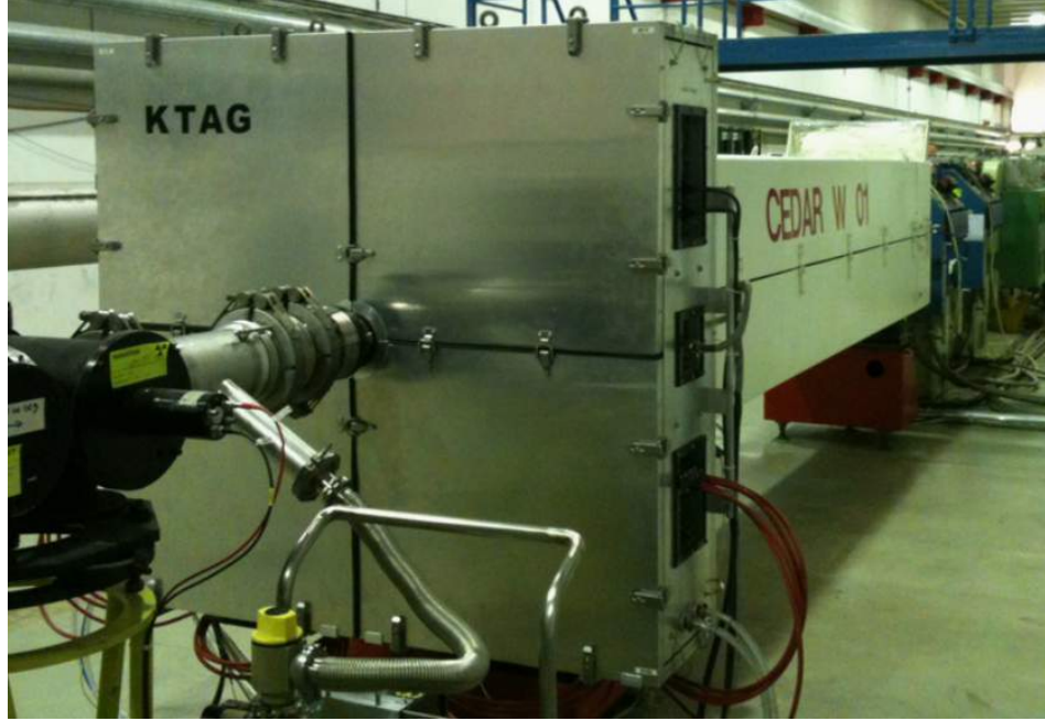
Figure 4.1: A picture of the CEDAR vessel and KTAG Detector in situ on the beam line.
