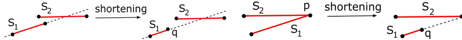
Fig. 9. Left: shorten a segment S_1 to the new endpoint q with d(q, S_2) = \text{Min\_Distance} . Right: shorten a segment S_1 away from S_2 to avoid a small angle \theta < \varphi between S_1, S_2 .
