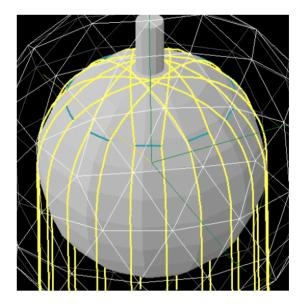
Figure 3.5: Visualisation of the hold-down rope system which compensates for the buoyancy of the AV due to the lower density of scintillator than water [84].
