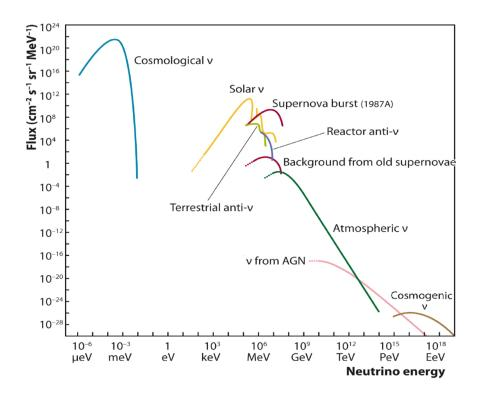
Figure 1.7: Neutrino flux at the Earth's surface [30].
