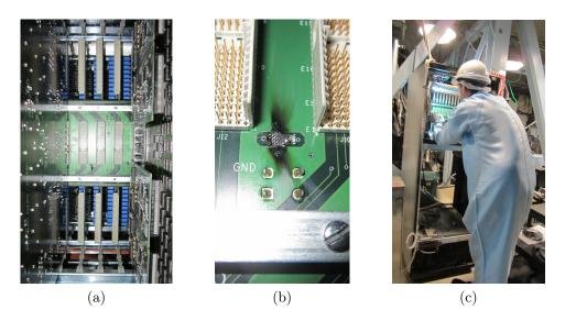
Figure 3.15: A backplane seen through the gap created by removing three FECs (a), a zoomed in shot of the damage caused by the blown capacitor (b), and this author replacing all capacitors on a crate (c).
