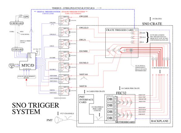
Figure 2.2: A block diagram of the SNO trigger system [86] which has been refurbished for SNO+. The XL3 boards which read out the charge and time information to the DAQ are not shown, and the MTC/A cards are replaced by MTC/A+.
