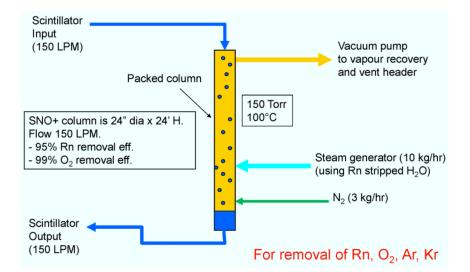
Figure 3.4: A flow diagram of the SNO+ gas stripping scintillator purification system. The stripping gas is a combination of nitrogen (3 kg/h) and super-heated steam (10 kg/h) [108].
