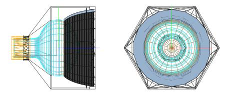
Figure 5.14: A visualisation of the SNO+ PMT geometry from the side (left) and top (right) [142].
