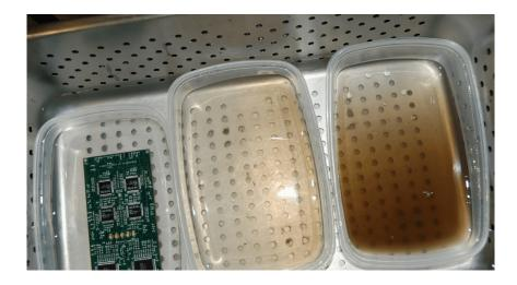
Figure 3.13: Photograph of dark matter being removed from the electronics circuitry [119].
