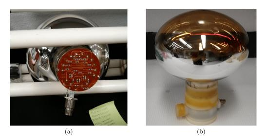
Figure 3.12: Exposed base circuitry of a PMT in repair (a) and a fully repaired and resealed tube (b) [115].
