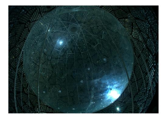
Figure 3.6: A photograph taken from below the acrylic vessel, showing the hold-down rope system [112].
