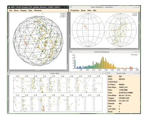
Figure 5.2: A visualisation of a typical flasher from SNO with the SNO+ event viewer. The histogram is of uncalibrated hit times defines the colours in the other windows.
