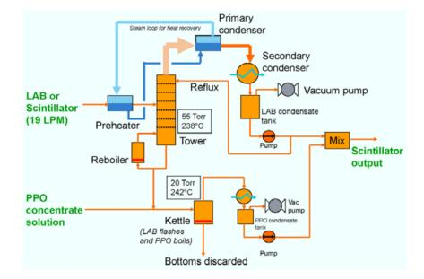
Figure 3.2: A flow diagram of the SNO+ distillation system. The distillation tower is used for vacuum distillation of LAB, while the kettle flash distills a concentrated solution of PPO in LAB. The tower can also distill scintillator for the recovery and purification of PPO [108].
