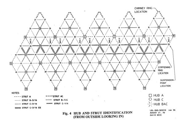
Figure 3.7: Flat map view of the detector with node panel numbering [113].
