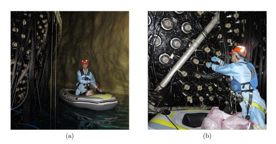
Figure 3.11: Boating in cavity (a) to access PMTs due to be replaced (b).
