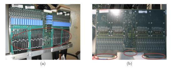
Figure 3.10: (a) The front face of a PMTIC, which connects the PMT cables (circled) to the electronics system. (b) The rear face of a PMTIC. The position of the connectors to the backplane and corresponding FEC are circled.
