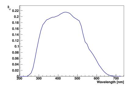
Figure 4.5: The quantum efficiency of the PMTs, defined as the probability of a photoelectron being liberated from the photocathode.
