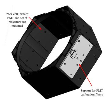
Figure 3.8: Mounting position for a TELLIE fibre plate [88].
