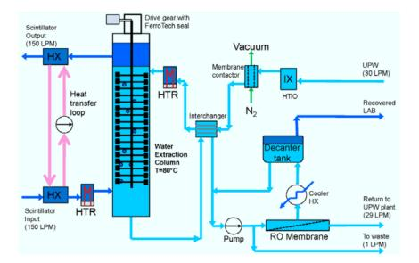
Figure 3.3: A flow diagram of the SNO+ water-extraction scintillator purification process [108].
