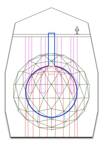
Figure 2.1: Diagram of the SNO+ detector showing the  $\sim 18$  m geodesic PMT support structure (green), housing a 12 m diameter acrylic vessel (blue). The AV is suspended by a system of high purity ropes (purple) and held down by a rope net (red). The AV and PSUP are contained in a volume of ultra-pure water [85].
