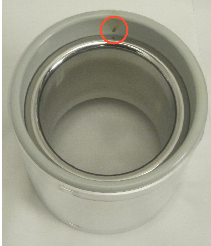
Figure 5.6: High-voltage barrier from SAGE. The stainless steel electrode is the central cylinder. It is surrounded by a Noryl resin insulator and an aluminium grounding sleeve. This is the barrier that had to be replaced in the second beam time and the black mark on the insulator (circled at top of picture) is probably from the barrier discharging by sparking. The outer diameter of the barrier is 146 mm.
