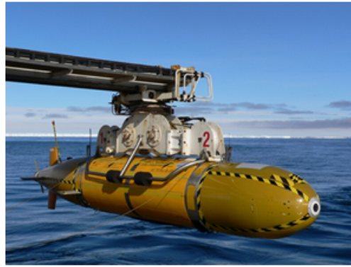
Figure 3.2: NOC Autosub 3 being deployed off the Pine Island Glacier
