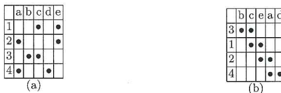
Fig. 1. Banding Example: (a) raw data (b) rearrangement of columns and rows to reveal a banding
