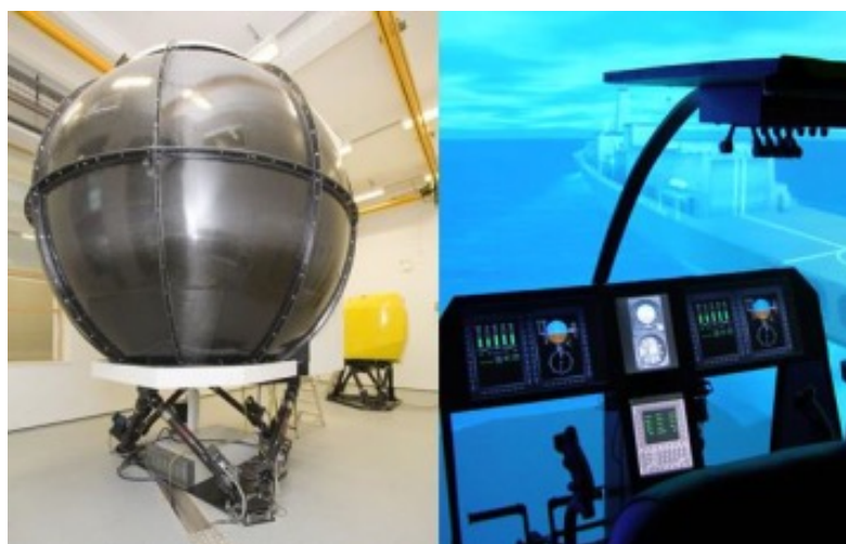
Figure 2 HELIFLIGHT-R simulator – internal and external views
