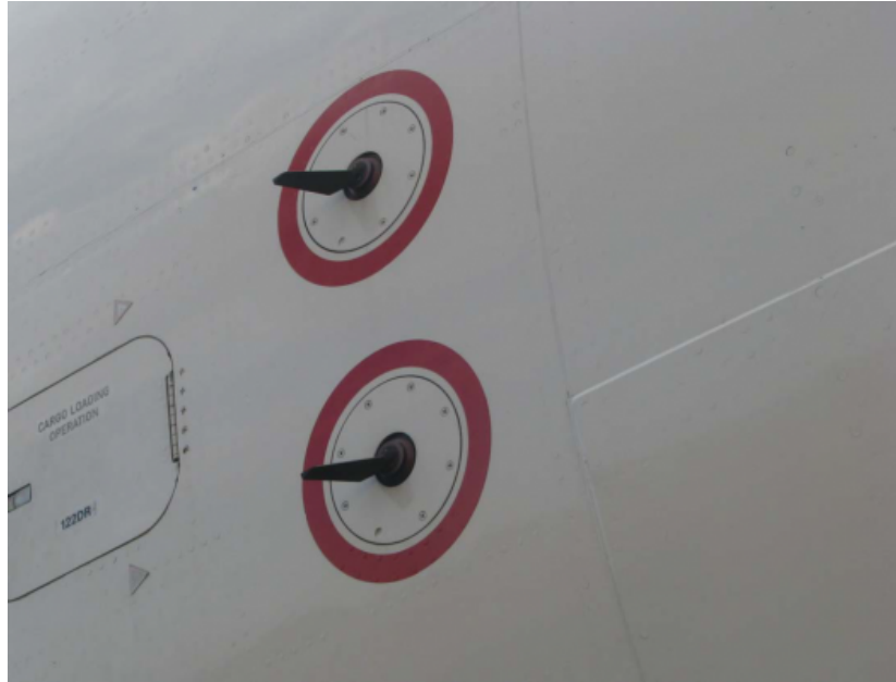
Figure 4.2: Two Angle-of-Attack Sensors on Airbus A330 [2]
