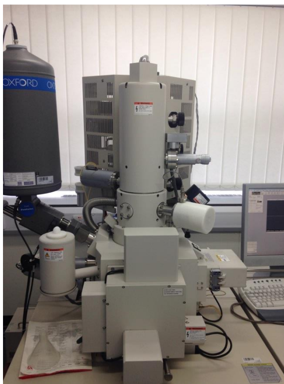
Figure 2.4 Image of Hitachi S-4800 Field Emission Scanning Electron Microscope used to determine morphology and particle size.
