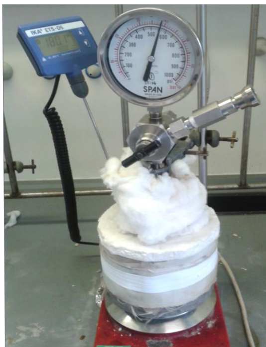
Figure 2.8 Image of the reactor setup used for preliminary experiments in Diels-Alder cycloaddition of 2,5-dimethylfuran (DMF) with ethylene.
