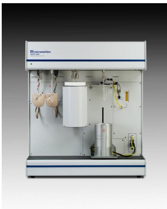
Figure 2.1 Image of Micromeritics ASAP 2020 used for specific surface area and porosity measurements.
