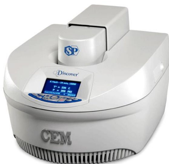
Figure 2.7 Image of CEM Discover SP used to synthesise various zeolites and the Friedel-Crafts alkylation of benzyl alcohol with benzene.
