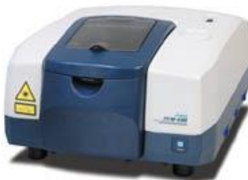
Figure 2.3 Image of Nicolet NEXUS FTIR spectrometer used to distinguish between Brønsted (B) and Lewis (L) sites.
