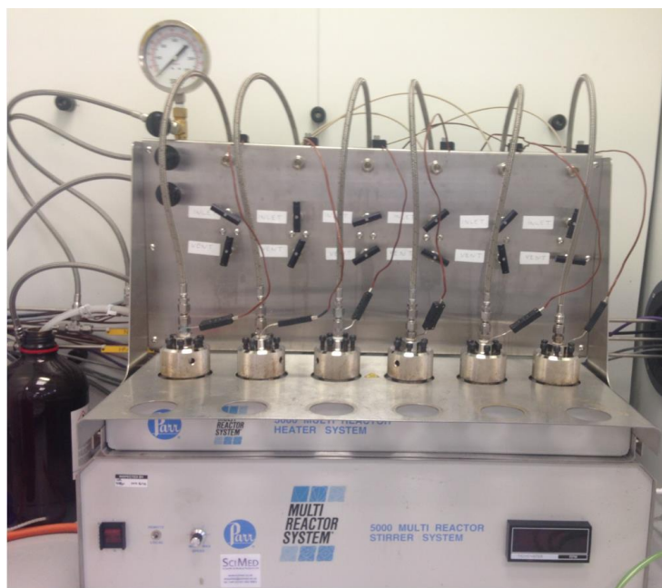
Figure 2.9 Image of the reactor used for the Diels-Alder cycloaddition of 2,5-dimethylfuran (DMF) with ethylene.
