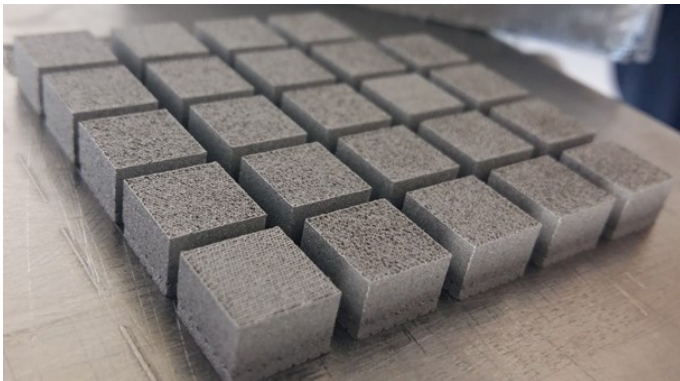
Figure 8: Tungsten components manufactured using SLM
