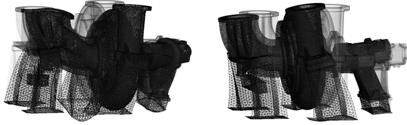
Figure 7: Mode shapes \phi_1(\mathbf{h}^1) and \phi_2(\mathbf{h}^1) for Pump 1.
