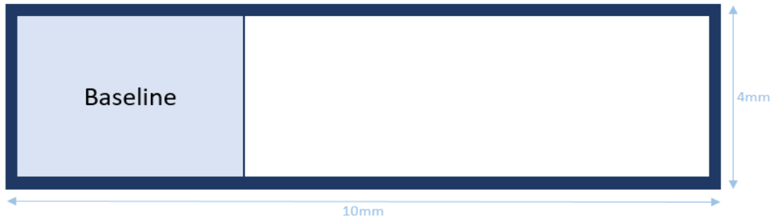
Figure 2.6: Preparation for Baseline Analysis. In order to keep an area for baseline analysis, one third of the experimental window was covered.
