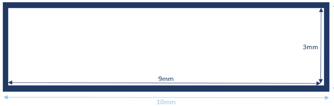
Figure 2.4: Schematic of Prepared Experimental Block. Illustration of fully prepared bovine enamel block with a 9x3mm experimental window on the polished surface.
