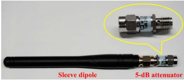
(a) AUT with a 5-dB attenuator
