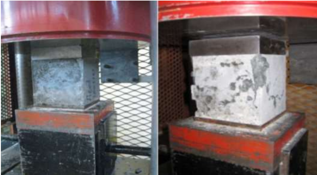
Figure 3.7: Cube positioned in the 3000 kN TONIPACK compression test machine.
