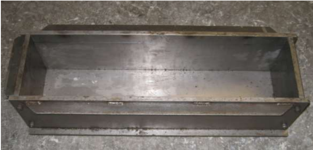
Figure 3.4: Steel mould for preparation of prismatic elements.
