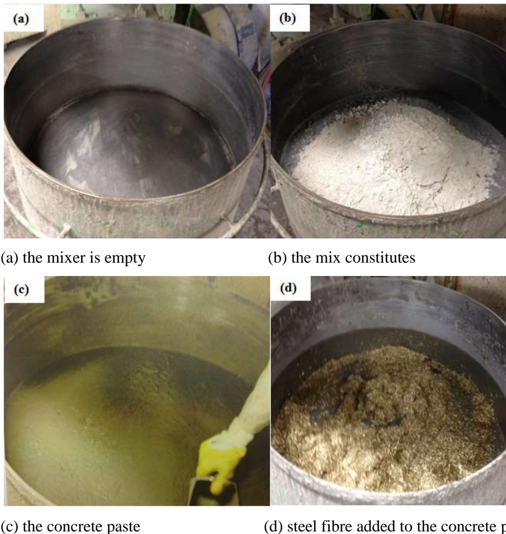
Figure 3.8: Mixing procedure of UHPFRC
