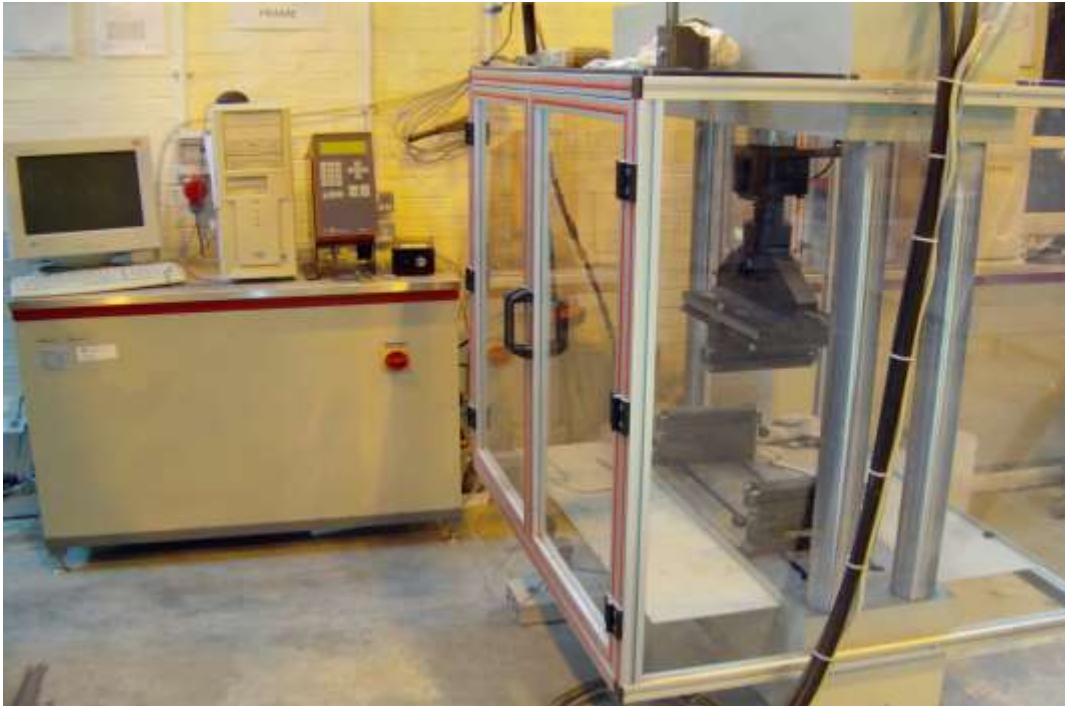
Figure 3.3: General set-up of Zwick test machine.
