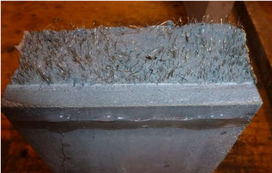
Figure 3.15: Fracture surface with pulled-out steel fibres.
