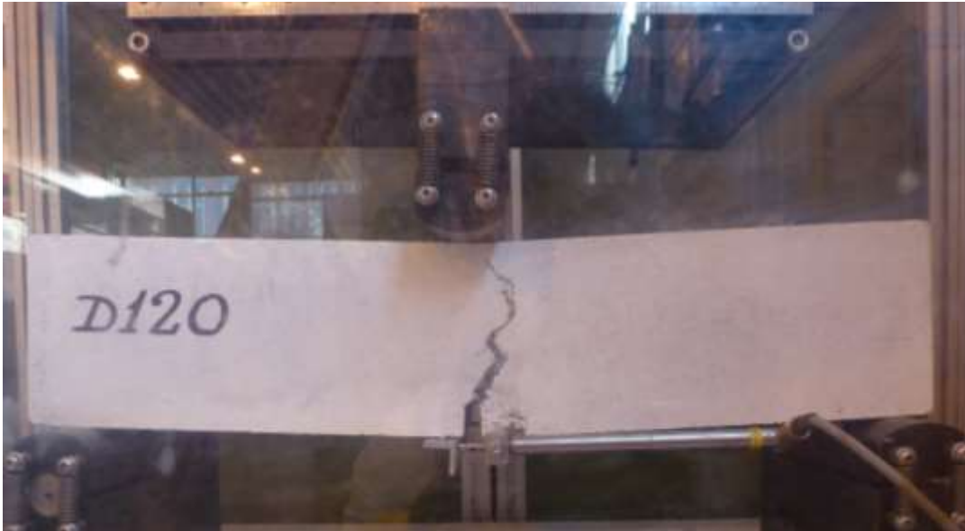
Figure 3.11: Test setup of notched 3-point flexure test of UHPFRC beams.
