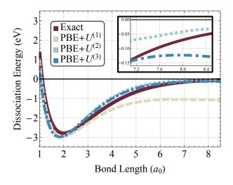
FIG. 3. (Color online) The  $H_2^+$  dissociation curves of the exact functional (solid), PBE+ $U^{(1)}$  (dashed), PBE+ $U^{(2)}$  (dotted), and PBE+ $U^{(3)}$  (dot-dashed). In the dissociated limit (inset), the  $U^{(2)}$  result tends asymptotically to the exact one, and the  $U^{(3)}$  scheme begins to deviate from it non-negligibly.
