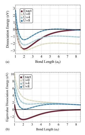
FIG. 1. (Color online) The dissociation energy curve of  $H_2^+$  calculated from (a) the total-energy and (b) the occupied Kohn-Sham eigenvalue using the exact xc-functional (solid), and PBE+U with U = 0, 4, 8 eV (dashed). PBE+U successfully resolves the SIE in the total-energy, for a strongly bond-length dependent Hubbard U, but it does not address the inaccuracy in the Kohn-Sham eigenvalue, or non-compliance with Koopmans' condition, which grows with bond-length.
