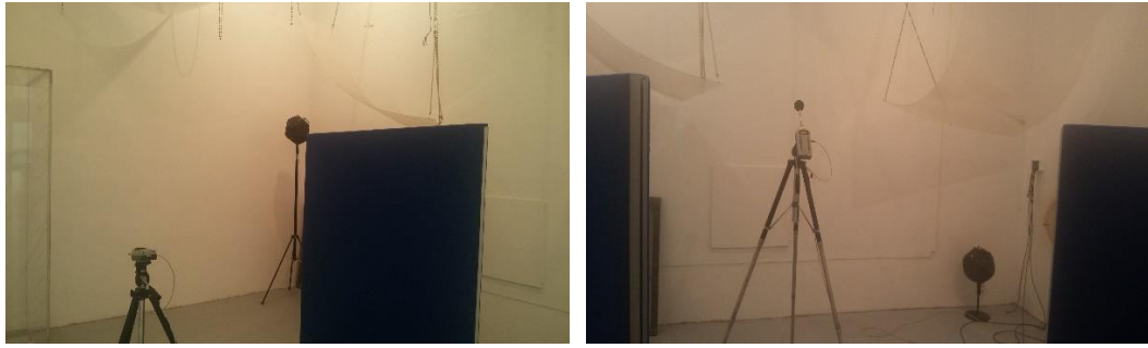
Figure 2-13. Measurement setup for the absorption coefficient of the partition used for the real corridor experiment in the reverberation chamber at two different position of the omnidirectional power source and with two partitions.
