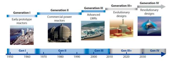
**Figure 2.** Generations of nuclear power: Time ranges correspond to the design and the first deployments of different generations of reactors [5].
