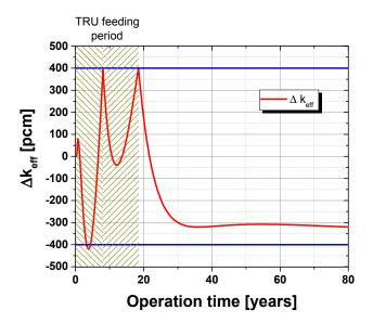
**Figure 5.** Change of the deviation of the averaged effective multiplication factor  $\Delta Keff$  over a simulated operational period of 80 years within the iteration band of  $\pm 400$  pcm.
