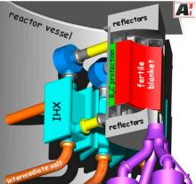
**Figure 10.** (**Right**): Simplified scheme of the MSFR system including the core, blanket and heat exchangers (IHX)—(**Left**): Benchmark definition [30].
