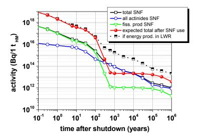
Figure 9. Activity per ton of SNF over time.
