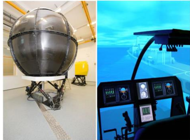
Figure 3 The University of Liverpool HELIFLIGHT-R motion base research simulator
