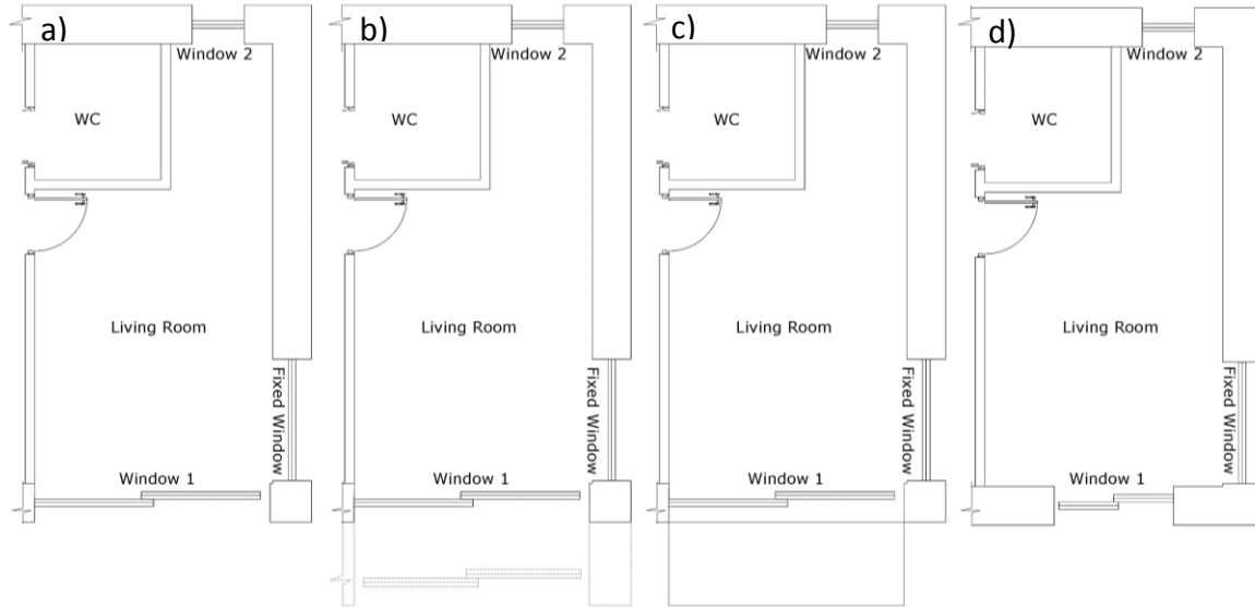
Figure 8-3 Living room plan and notation of the investigated representative rooms; a) original case study, b) tilted façade, c) overhang, and d) 26% WWR
