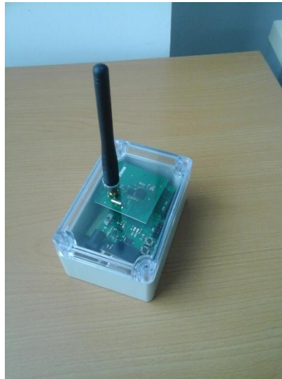
Figure 26: CC2430 covered by a box
