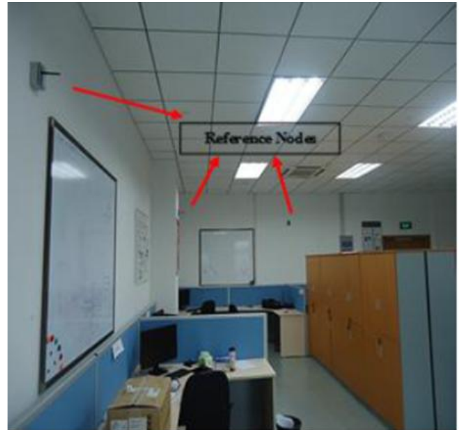
(b) Fixed reference nodes installed in an office
