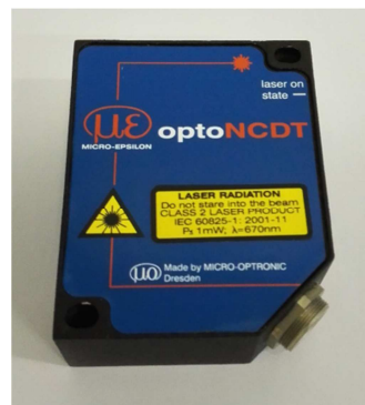
Figure 5.5. Laser transducer used to measure displacement
