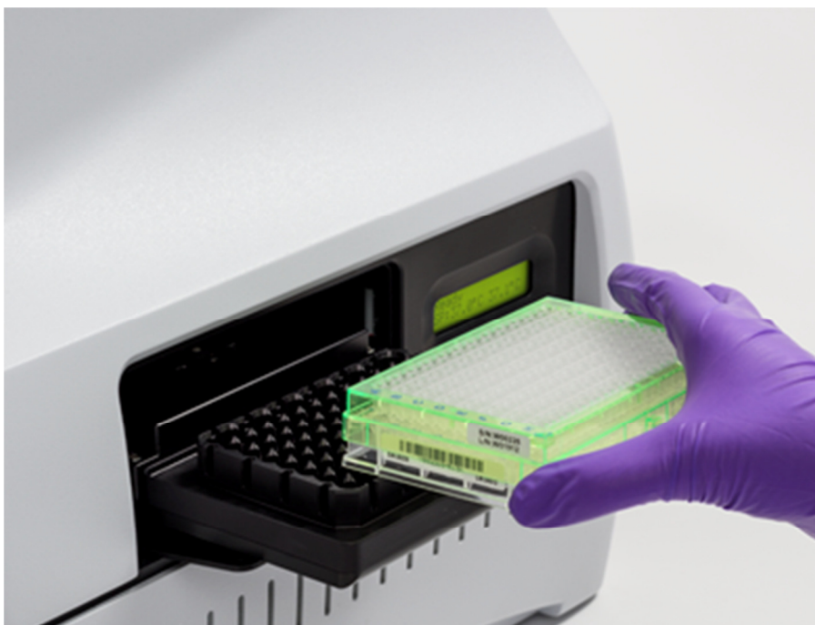
Figure 2.6. Seahorse XFE96 Bioanalyser with the florescent sensor-containing cartridge (green) sitting above the culture plate (white).
