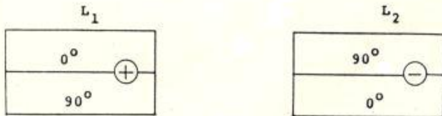
c) Cross-ply Laminated System in its Simplest Shape (⊕ and ⊖ indicate the sign of B_{11} )
