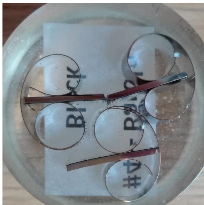
Figure 6.12: Dissected automotive samples, which are fixed and resin-mounted. The cross-sections of samples are carefully polished and placed upwards in order for microscopy imaging.
