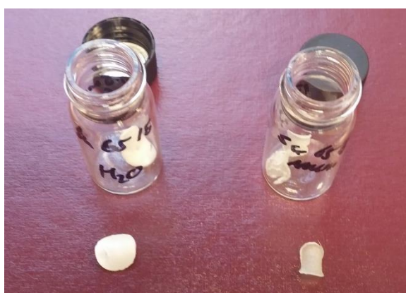
Figure 8.2: Freeze dried hydrogel after water washes (left) or NMM washes (right).
