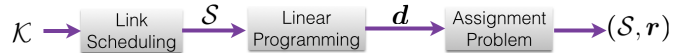
Fig. 4: The separated solution with a heuristic link scheduling and assignment-based power control, where the desired GDoF tuple is obtained via linear programming over the selected convex polytope.
