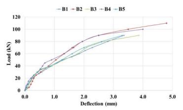
Fig. 3. Load-deflection curves for NSC T-beams prior to failure.
