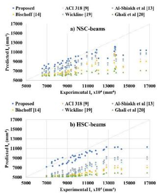
Fig. 5. Comparison between different equations for predicting I<sub>e</sub> values of a) NSC and b) HSC T-beams.
