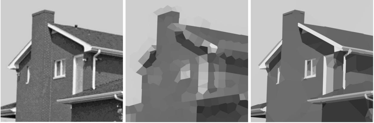
Fig 2 Left: input. Middle: 275 Voronoi cells, 5 nRMS \approx 10.2\% . Right: 246 CCM superpixels, nRMS \approx 4.48\% .
