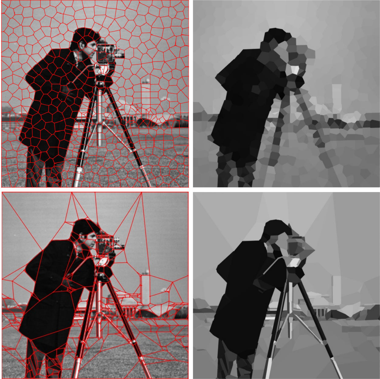
Fig 4 Top: 589 Voronoi superpixels (boundary mesh and reconstructed image) have nRMS \approx 9.22\% . Bottom: 416 CCM superpixels (boundary mesh and reconstructed image) have the smaller error nRMS \approx 6.32 from Definition 9.
