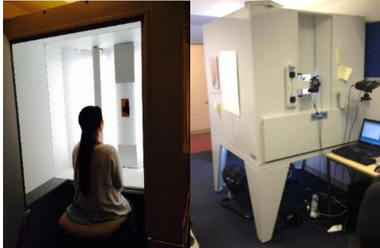
Figure 3. The subject sitting in the front of the viewing cabinet (left) and the telespectroradiometer mounted at the back of the viewing cabinet (right).
