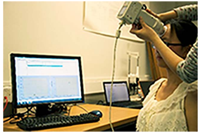
FIGURE 1 The spectrophotometer location to obtain measurements on the subject's forehead
