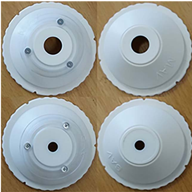
FIGURE 2 The four masks used to make measurements using the spectrophotometer. Upper left: medium aperture/low pressure (MA/LP). Lower left: small aperture/low pressure (SA/LP). Upper right: medium aperture/high pressure (MA/HP). Lower right: small aperture/high pressure (SA/HP)
