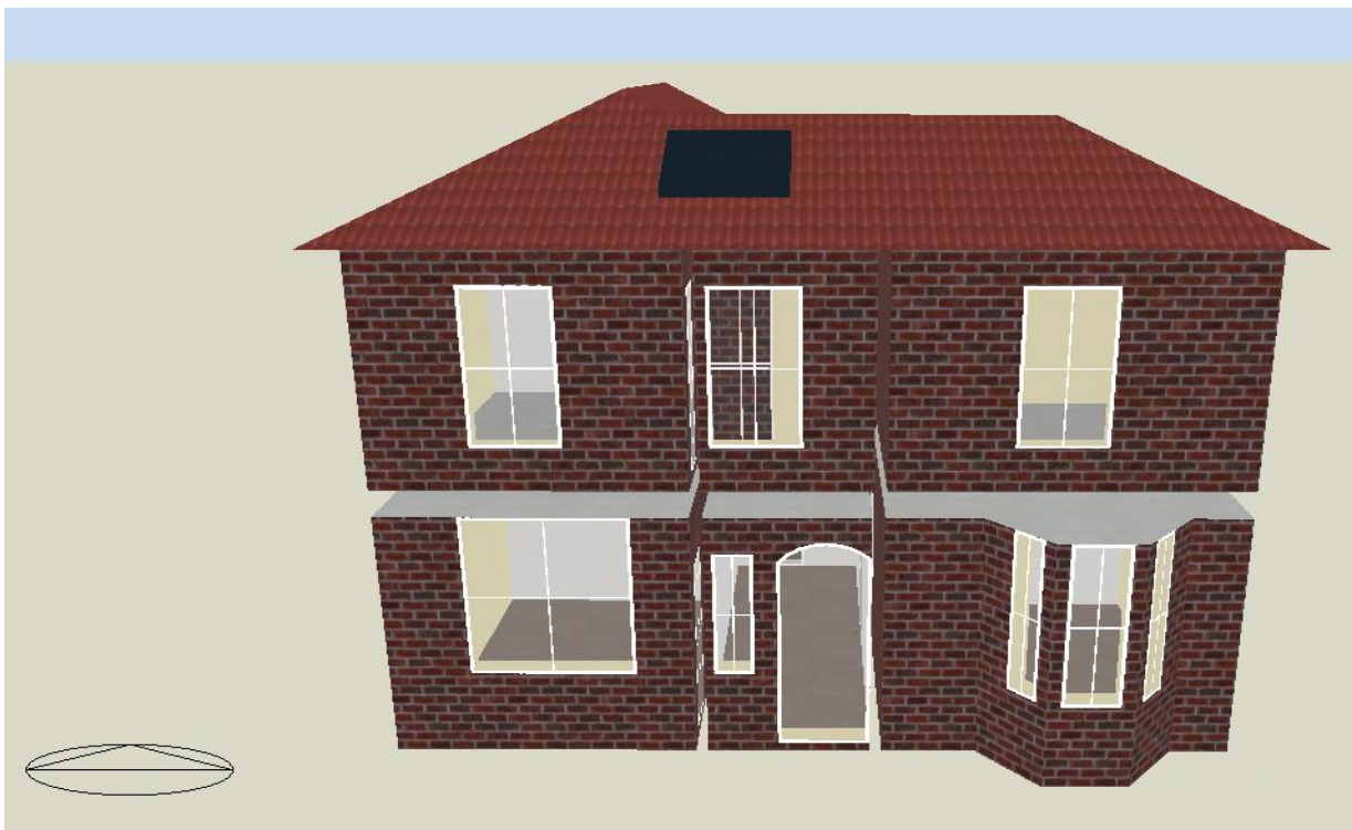
Figure 0:1: Exported gbXML file into DesignBuilder through native option of gbXML in ArchiCAD 20
