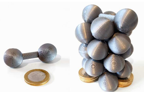
Fig. 1 A helical stack of ten 3D-printed dumbbells with D_{\infty h} symmetry. The dumbbell second from the bottom is supported by two stacks of coins to keep the helical stack upright.
