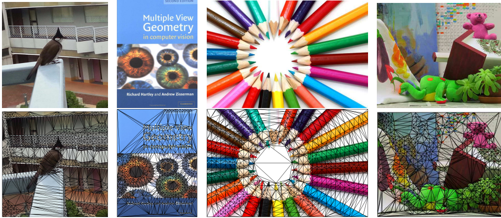
Figure 7: Several images and the triangulations by our TRIM algorithm. Top: the input images. Bottom: the resulting triangulations. The key features of the images are well represented in our triangulations, and the regions with similar color can be represented by coarse triangulations.
