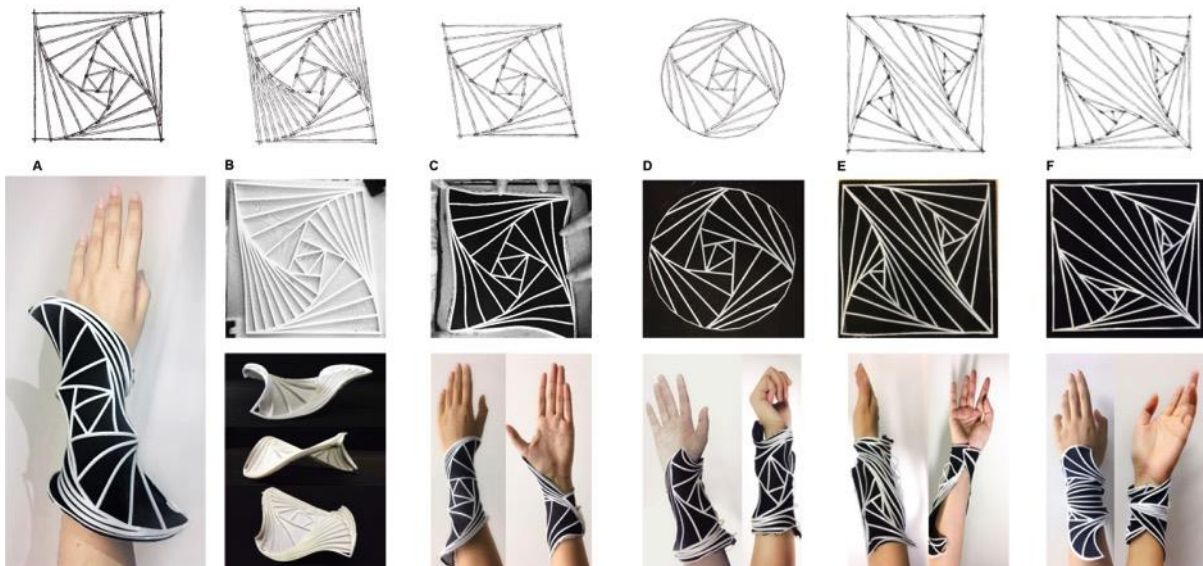
Figure 4: Tests A, B, C, D, E, F - Two directional embossed patterns calculated to produce a wearable with prescribed form
