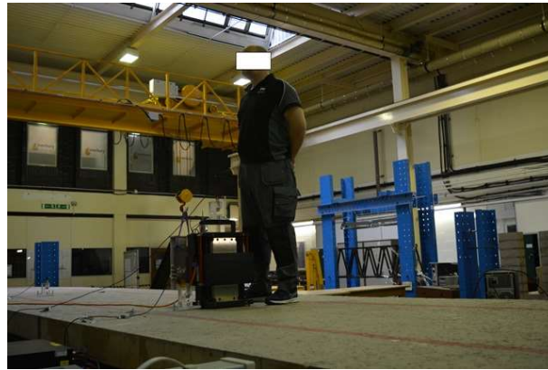
Fig. 7 The bridge with the shaker and the human occupant at TP1
