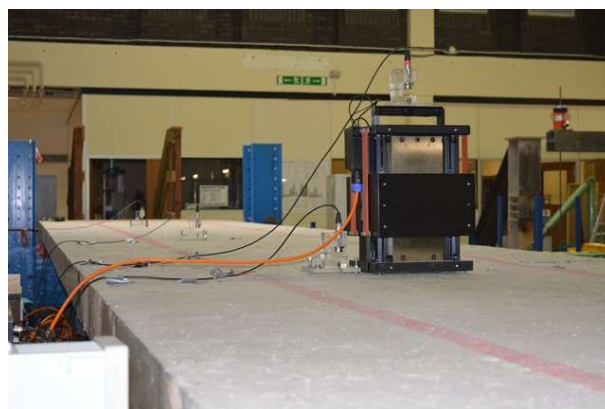
314 Fig. 5 The bridge with the shaker at TP1
