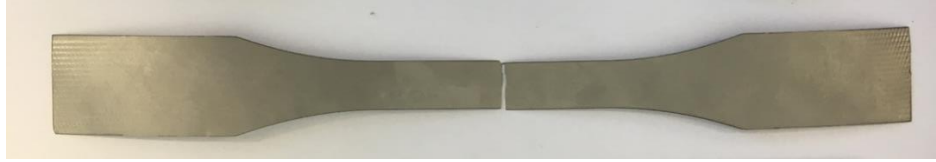
Figure 4-39. Typical failure mode in the titanium alloy specimens following tensile testing.
