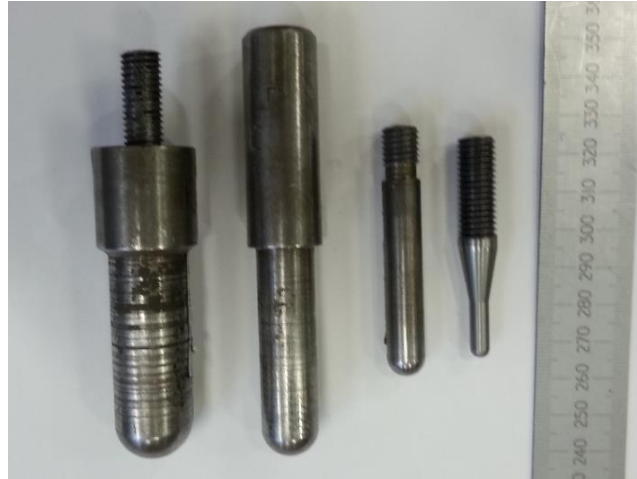
Figure 3-14. Hemi-spherical projectiles with diameters of 5, 10, 15 and 20 mm.
