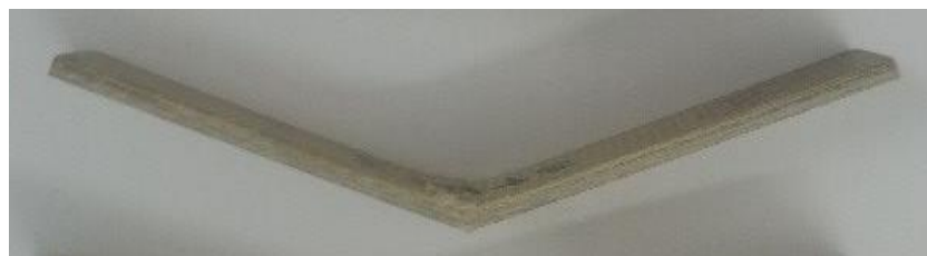
Figure 4-11. Typical failure modes of the failed specimens under three-point tests.
