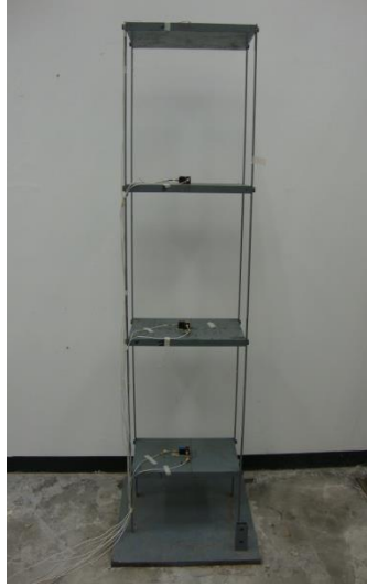
Figure 4. Shear frame in the laboratory
