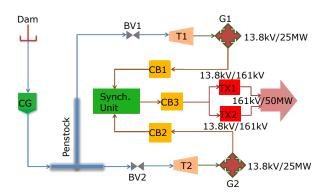
BV1: Butterfly Valve 1 CB1: Circuit Breaker 1 CG: Control Gate
