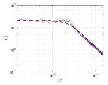
Figure 5: Gain of the transfer function from base moment to disk inclination, for the disk free to rotate: (—) measurements and (- -) oscillator model (19).
