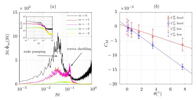
Figure 2: Premultiplied power spectra (inset: power spectra) of the azimuthal modes on the base of the fixed disk at  $\theta = 0^{\circ}$ . Mean moment coefficient (b) measured with the fixed disk (symbols and solid lines) and the free disk (dashed lines) produced by the base and front side of the disk. Each vertical line has the standard deviation in length.
