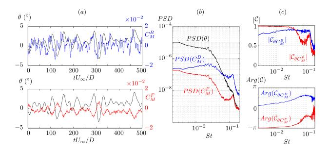
Figure 4: (a) Time signals of the disk inclination and front and base moments. (b) Power spectral densities. (c) Coherence functions (magnitude and phase) between inclination and moments.
