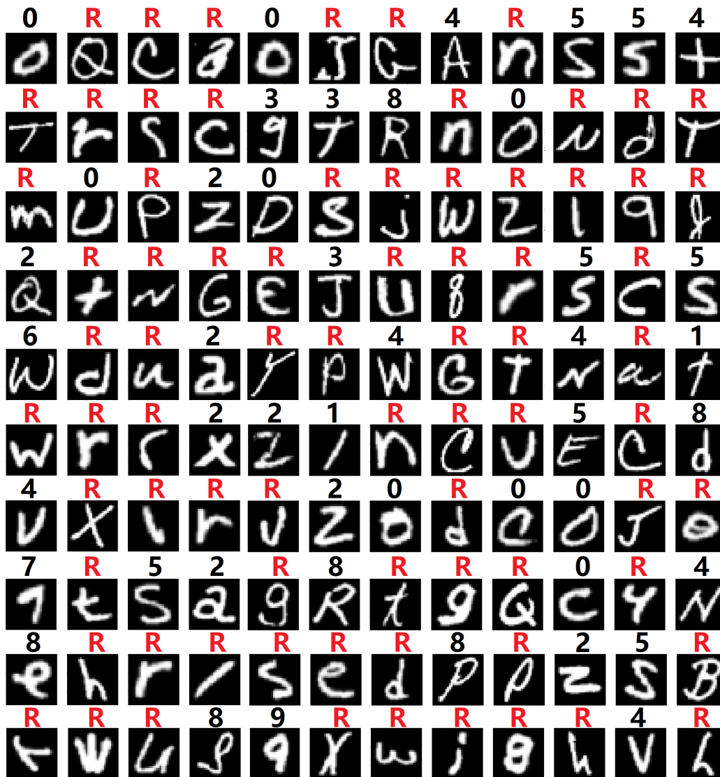
Fig. 6.6: Rejection results of 120 handwriting letters. The red R denotes the rejected results.
