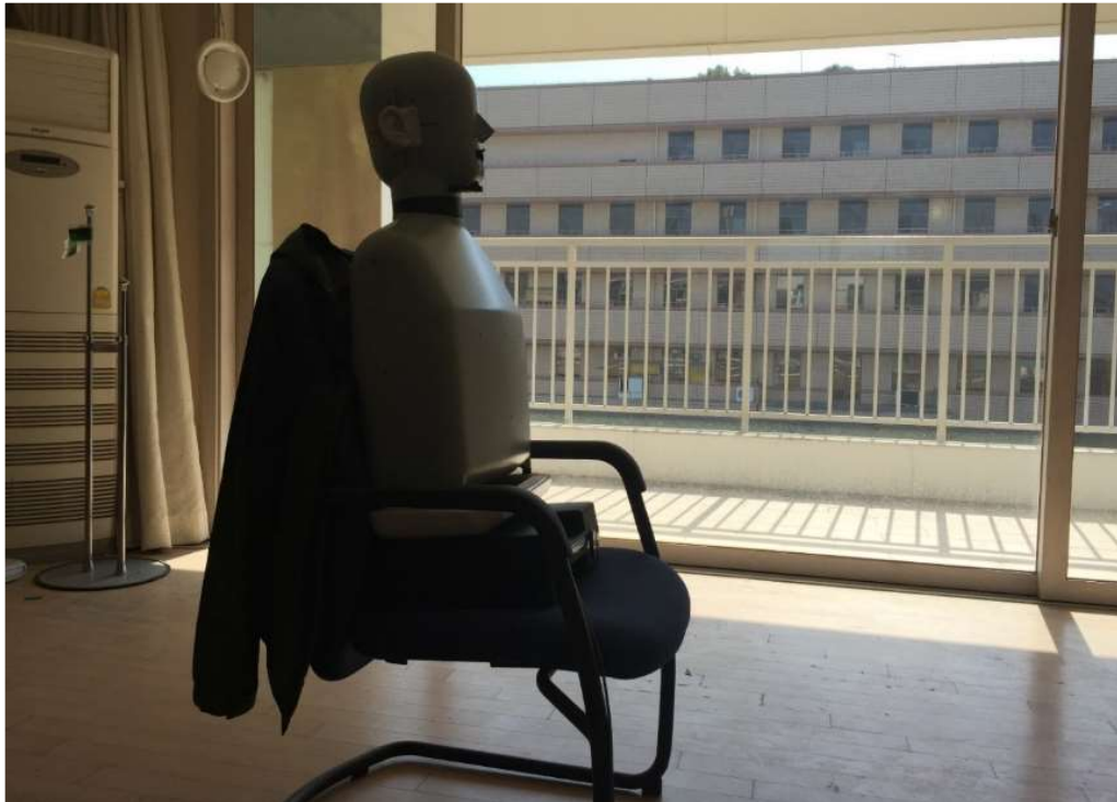
Figure A2-2. A head and torso simulator located in the receiving room (downstairs).
