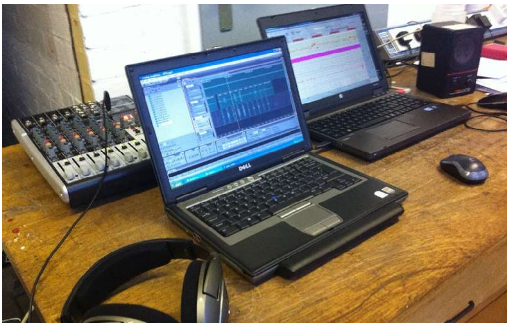
Figure A2-3. Outside of the audiometric booth: computers for stimuli presentation and data acquisition.
