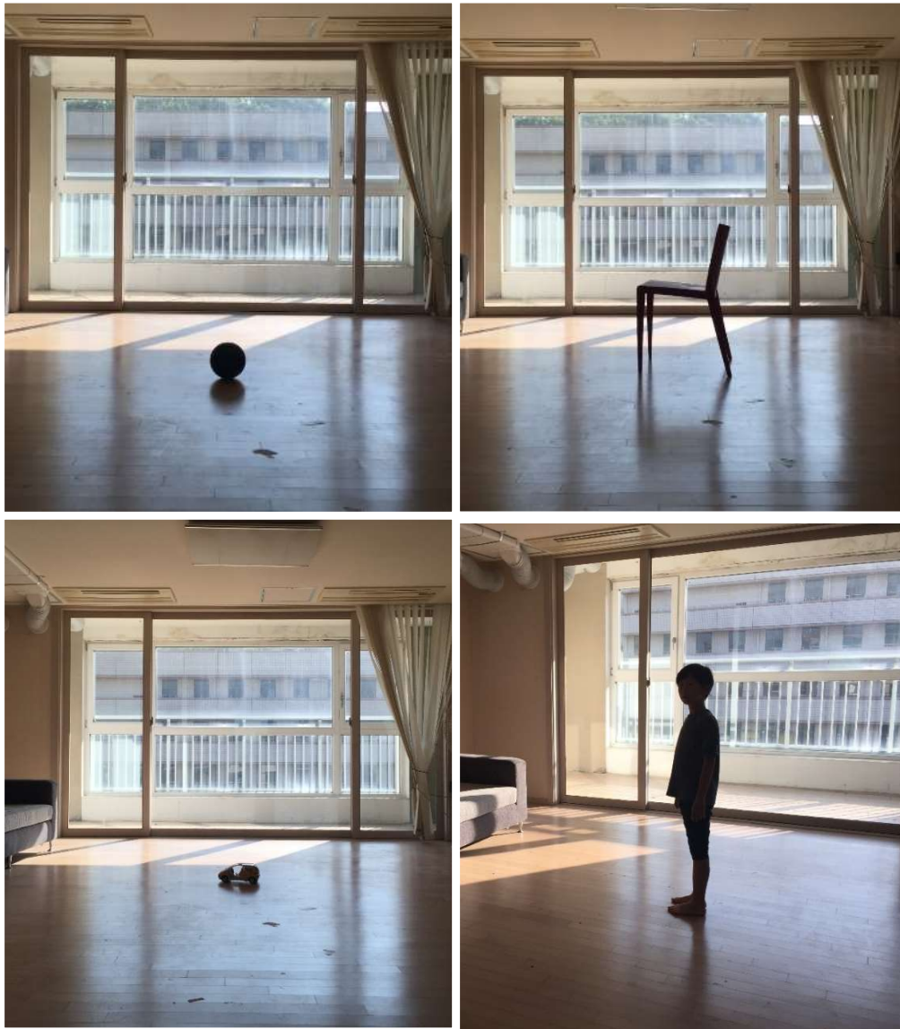
Figure A2-1. Noise sources in the source room (upstairs): an impact ball (top left), a chair (top right), a toy (bottom left), and a child (bottom right).
