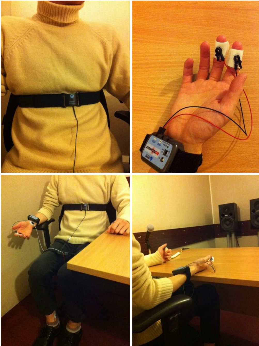
Figure A2-4. Electrodes were attached to the participant; the participant was seated in the audiometric booth and the loudspeakers were located in front of the participant.
