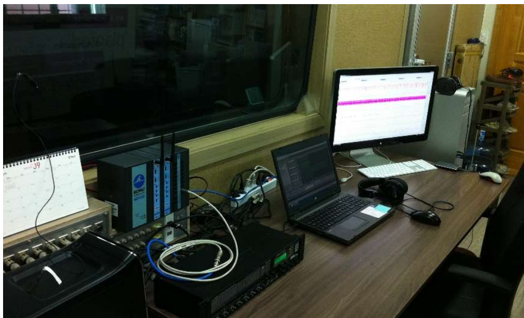
Figure A3-2. Outside of the audiometric booth: wireless amplifiers for physiological data recordings, computers for stimuli presentation and data acquisition.
