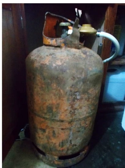
Figure 10 Example of poor-quality LPG cylinder (P3, F, age 28, Peri-urban, Income 1)
