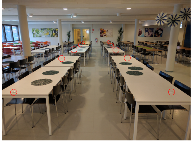
Figure 4: Scenario of the experiments. Ten beacons are placed on tables in a canteen at Aalto University. To aid visualisation, beacons are marked by a red circle.
