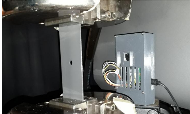
Figure 1: Experimental setup to monitor crack propagation
