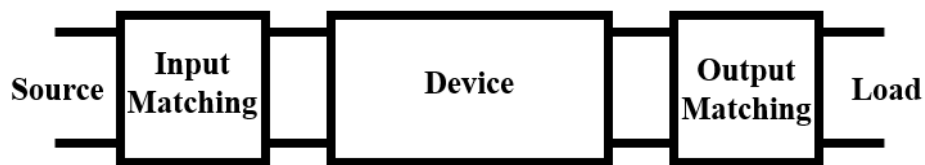
Fig. 1-2. General two-port network with matching units.
