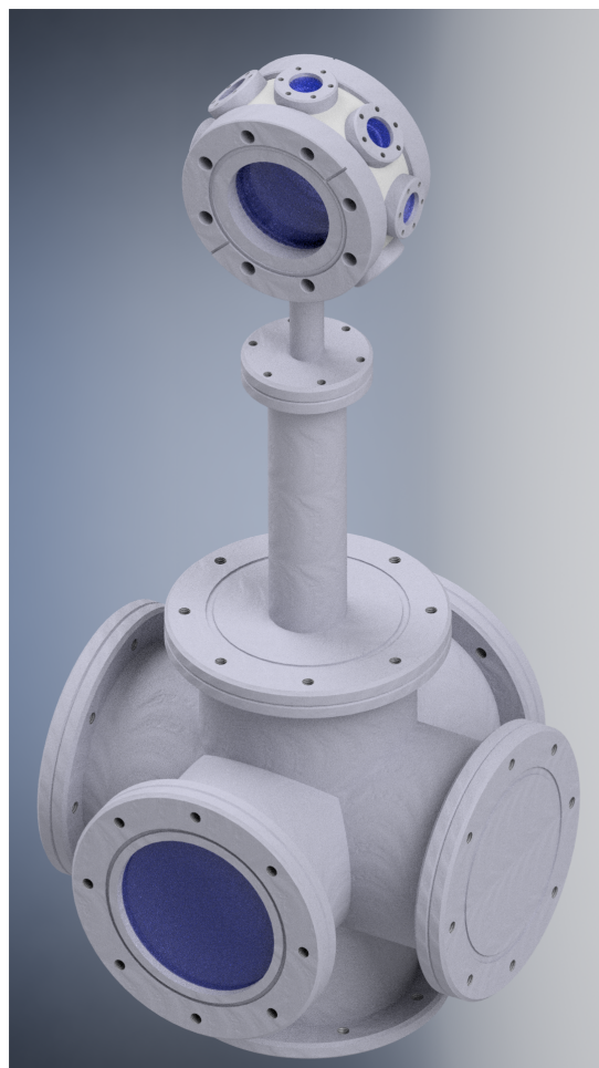
Fig. 3.1 Diagram of the current atom interferometry vacuum chamber, showing both the upper chamber for magneto-optical trapping and state preparation and the lower chamber for state detection.
