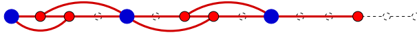
Figure 1: A 1-dimensional line of sight network ( n = 15 and \omega = 4 ). The dashed part represents \mathbb{Z}_{15}^1 . The big dark vertices form a maximum independent set.
