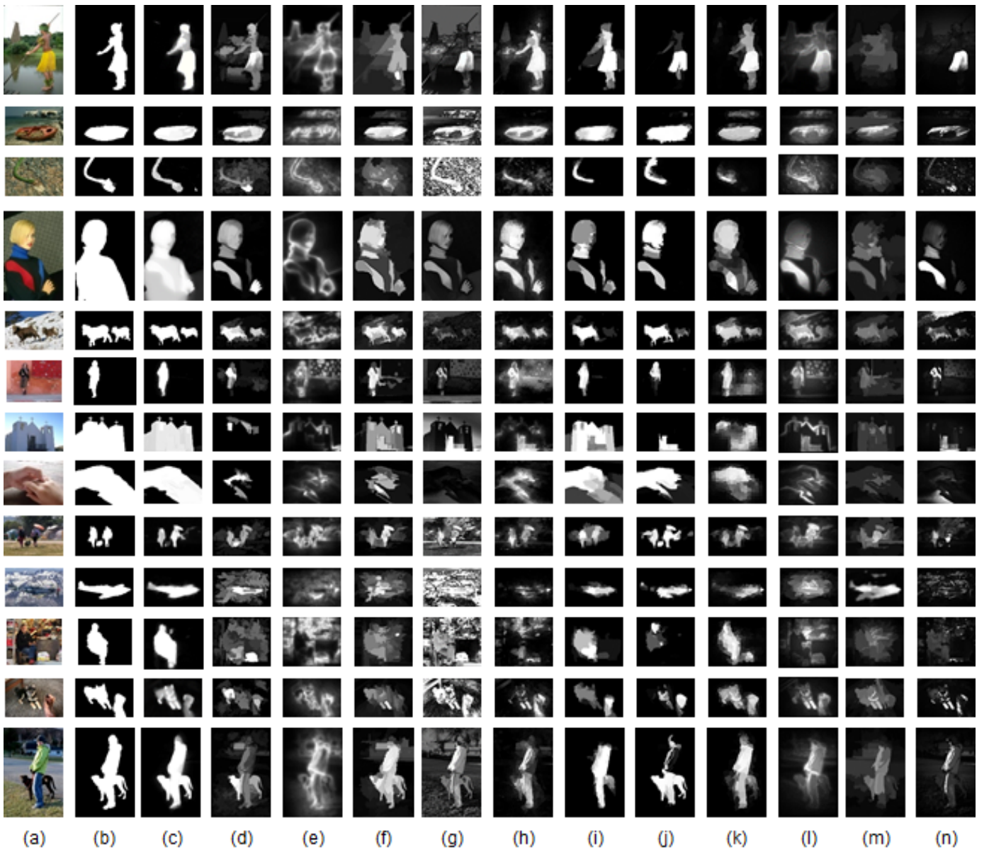
Fig. 6. The visual comparison of different salient object detection baselines. From left to right: (a) Original images, (b) ground truth, (c) our SP method, saliency baselines with (d) boolean map (BMS), (e) context-aware (CA), (f) discriminative regional feature integration (DRFI), (g) frequency-tuned (FT), (h) high-dimensional color transform (HDCT), (i) local estimation and global search (LEGS), (j) multiscale deep features (MDF), (k) multi-task deep saliency (MTDS), (l) principal component analysis (PCA), (m) contrast (RC), (n) saliency filters (SF).
